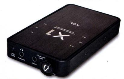
24-bit/192kHz sampling. Internally, the X1 has reference-quality components, including a gold-plated circuit board and connectors. It also has an internal rechargeable battery charged via the USB port.
